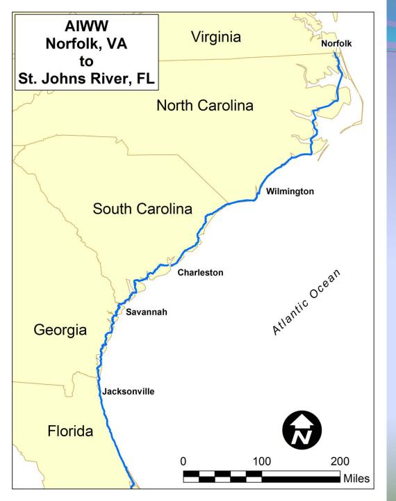
The Atlantic Intracoastal Waterway is a continuous sheltered waterway used by commercial and private shallow draft vessels. The **US Army Corps of Engineers maintains the** Waterway for 1,088 miles between Norfolk, Virginia and Miami Florida. The AIWW is authorized to 12 feet deep with widths of 90 feet through land cuts and 150 feet in open water areas.
