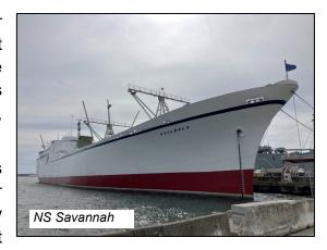
exceptionally quickly, with such low construction and operating costs that they were considered to be expendable in the course of war. The *Savannah* was built to demonstrate and test the practicality and safety of nuclear-powered vessels in commercial service.
